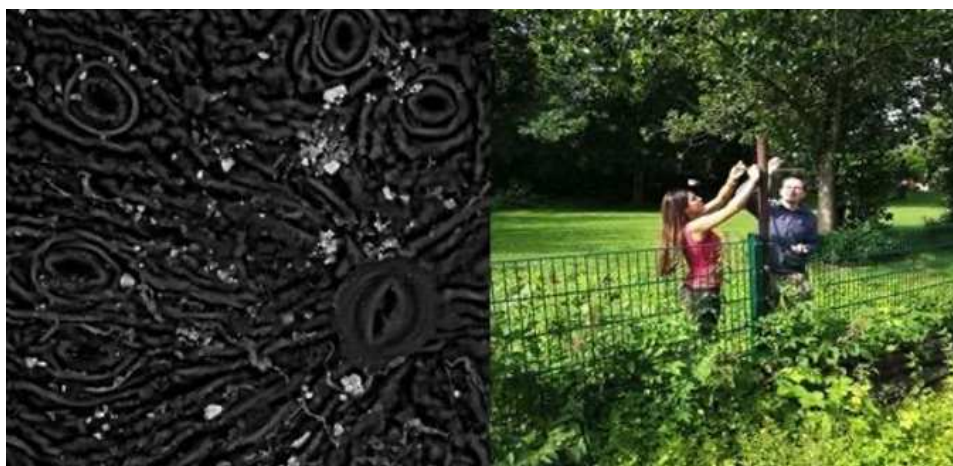
Figure 29. NBS characterised by the use of vegetation are highly effective for air pollution mitigation either in the case of particles deposited on the leaves and of gaseous compounds mainly absorbed through stomata. Left: Examples of Scanning Electron Microscope (SEM) images to detect morphology of leaves, number and quality of particles and stomata properties. Right: passive samplers installed in Dortmund to determine the role of NBS in air pollution mitigation. Source: PROGIREG project. Photo: G. Sgrigna and G. Guidolotti).
