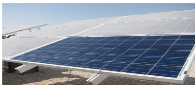
Figure 1. PV system after one month of soiling at the Qatari QEERI Solar Test Facility [4].
