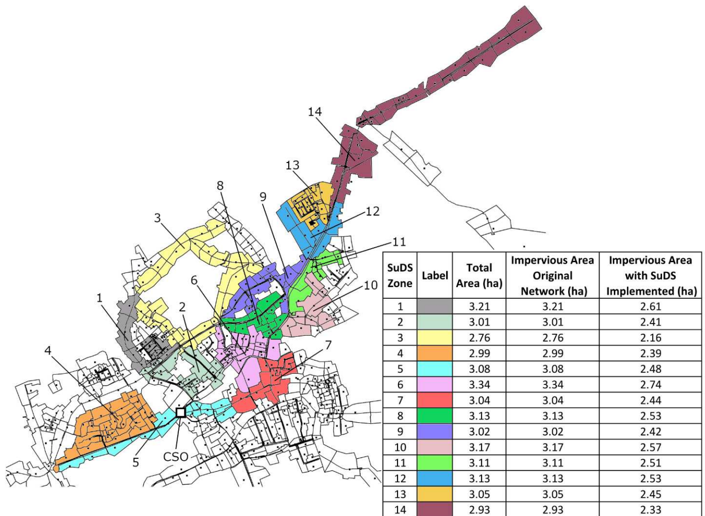
Figure 1. SuDS zones selected within the SWMM Arendonk sewer network model (0.6 hectares of impervious area were converted to pervious area in each SuDS zone).
