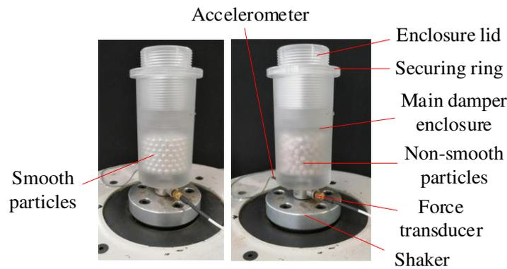
Figure 8 – Granular energy dissipation measurement rig with smooth and non-smooth particles.
