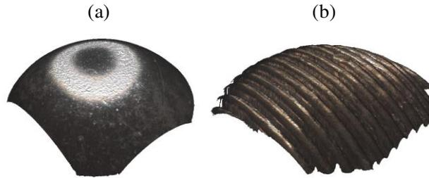
Figure 2 – Particle surfaces: (a) smooth and (b) non-smooth.
