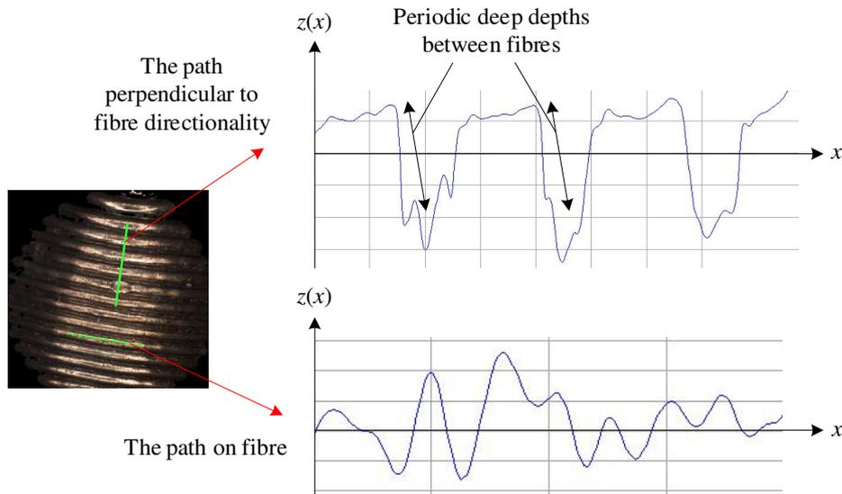
Figure 3 – Demonstration of different path directions on the non-smooth particle.
