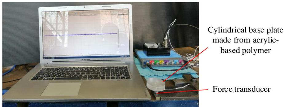
Figure 4 – Simple drop test rig.
