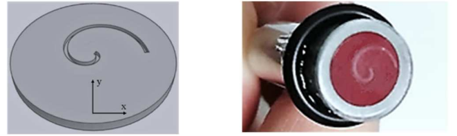
Fig. 3. (Left) 3D drawing of the acoustic lens with a spiral-shaped mask. (Right) Photograph of the transducer with the attached acoustic lens.
