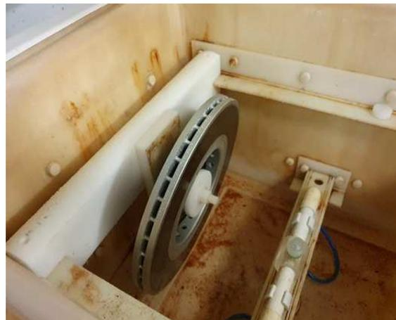
Fig. 2. Salt spray cabinet housing a brake disc
