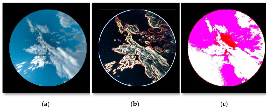
**Figure 4.** Evaluation of the proposed cloud decision algorithm: (a) Normal image captured using the full-sky imager, (b) the quaternion values of the image, (c) output image of the CA algorithm (blue–green color ratio); the back area represents CCF ratio = 1.0, blue area represents sky-free, and green is partial clouds.
