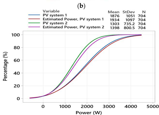
**Figure 10.** Output results when using the algorithm with PV systems: (a) output estimated power vs actual measured power in the examined PV systems (03 August 2022), (b) TSI image taken at 12:00, and (c) CDF distribution plot of the data taken from (a).
