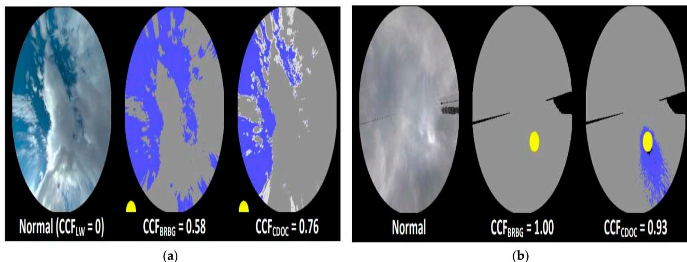
**Figure 3.** Evaluation of the CCF ratio for the BRBG and CDOC algorithms under two different shading conditions (note, the yellow circle represents the actual position of the sun in the sky, and the “normal” is the actual image captured using the full-sky imager): (a) partial shading, (b) overcasting.
