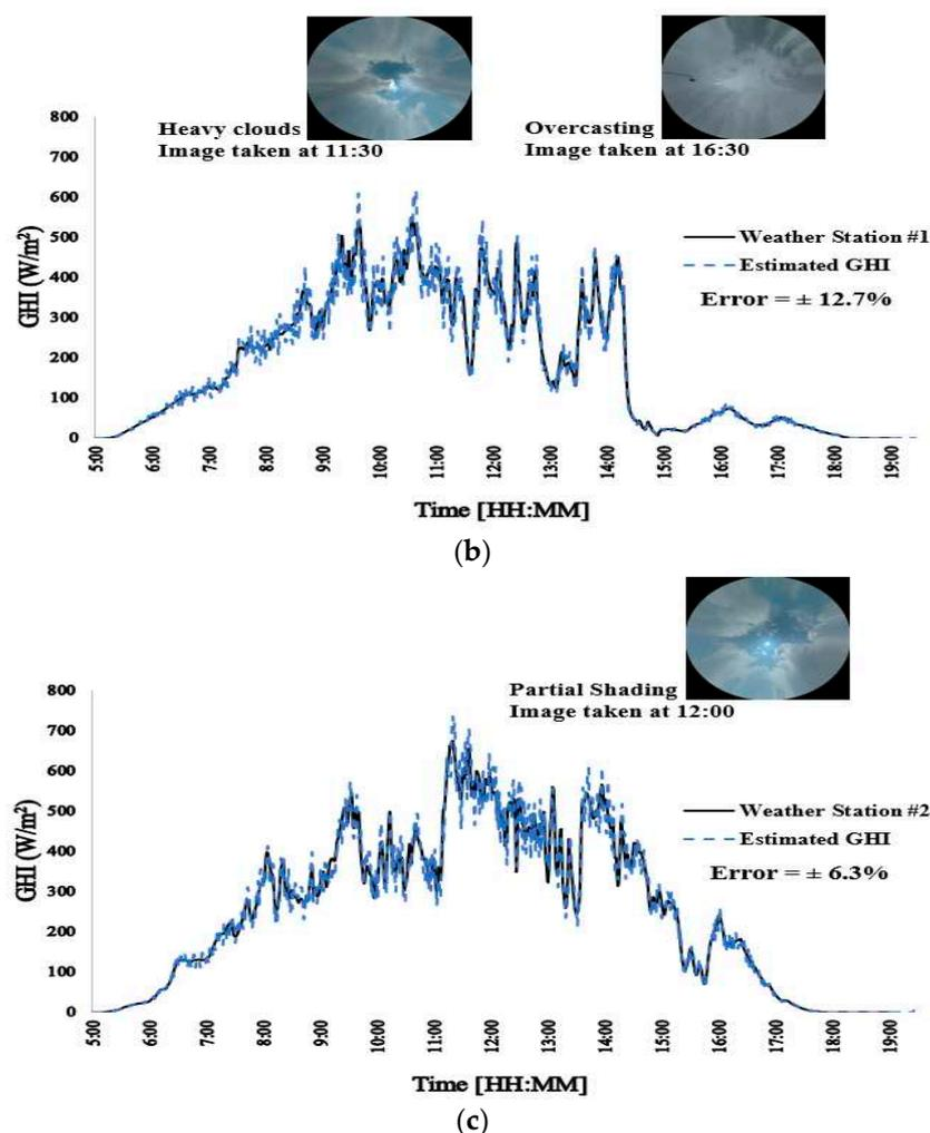
**Figure 7.** Output results of the estimated vs actual weather station GHIs under different shading conditions: (a) partial shading and clear sky, taken from weather station #1 (21 July 2022), (b) over-casting (heavy clouds), taken from weather station #1 (22 July 2022), and (c) partial shading, taken from weather station #2 (23 July 2022). (The sky images were taken from the nearest TSI, TSI-A for weather station #1 and TSI-D for weather station #2).
