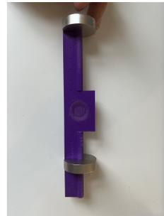
Figure 5 shows a 3D printed object with very little mass (around 2g), to which masses can be added along its length.
