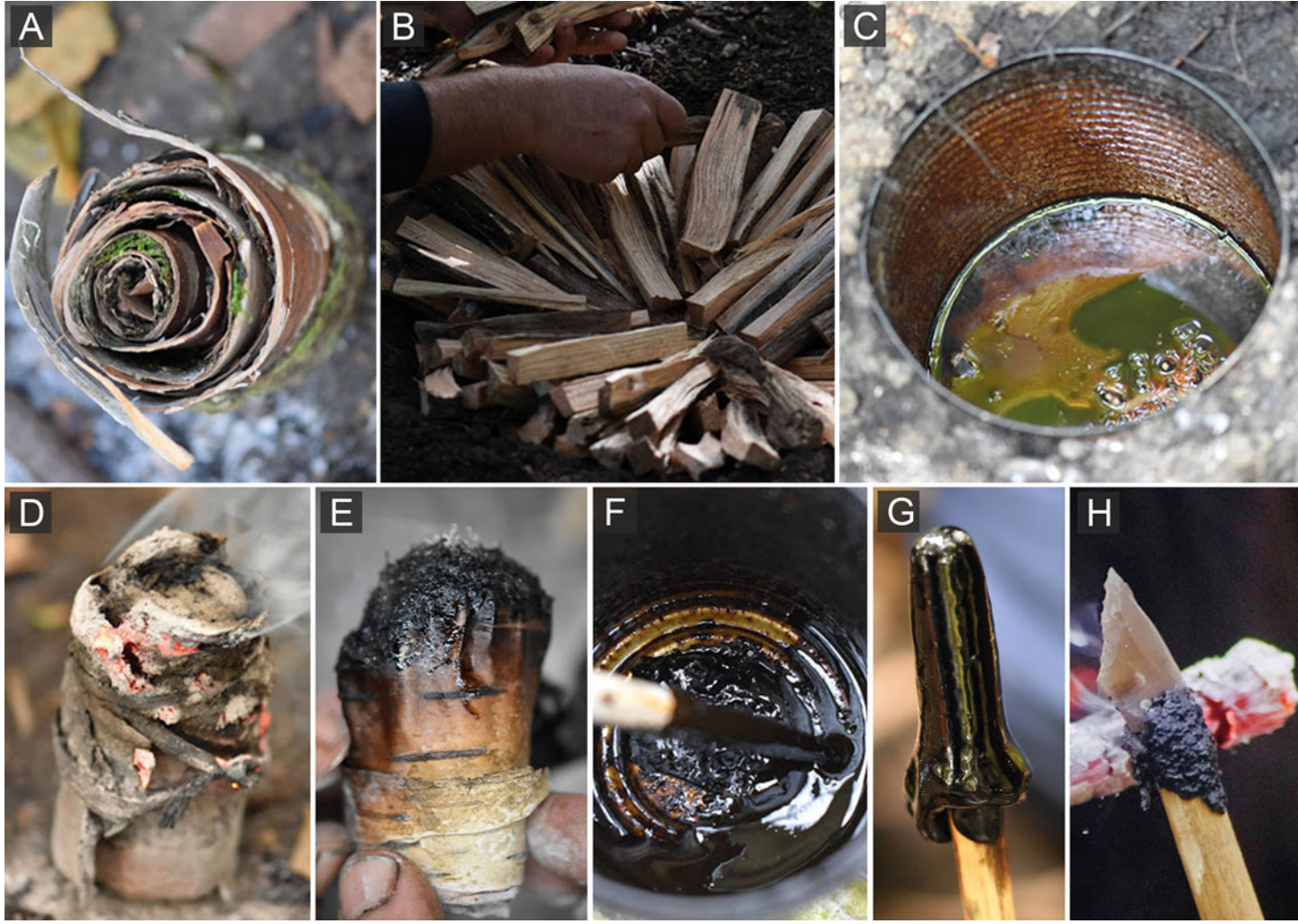
Figure 1. (A) Rolled birch bark; (B) aceramic pine-tar production; (C) aceramic yield of pine tar stored in a metal container post-production—turpentine, one of the pyrolysis fractions of pine wood, displays iridescent ‘rainbow’ effect; (D) roll of birch bark still burning post-use in aceramic production of birch tar; (E) birch bark undergoing phase-change from solid to liquid; (F) reflective and glossy yield of aceramicly produced birch-bark tar stored in metal tin; (G) a tar stick—useful for storing, transporting and reheating tar; (H) tar on a projectile is heated to make it malleable for moulding into desired form. (All photos © YEAR Centre.)
