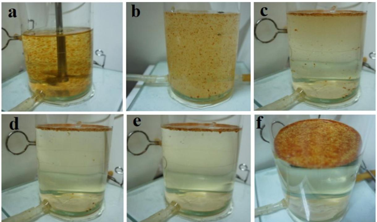
Figure 4: Photographs of different stages of  $\text{Fe}(\text{OH})_3$  precipitation, before and after flotation with MBs and NBs: (a) Precipitation; (b) Injection of MBs and NBs (c) Flotation at 30 s (d) Flotation at 1 min (e) Flotation at 5 min (f) Floated precipitates and treated water. Conditions  $[\text{Fe}^{3+}]_{\text{feed}} = 30 \text{ mg/L}$ ;  $\text{pH} = 7$ ; saturation time= 30 min [27].
