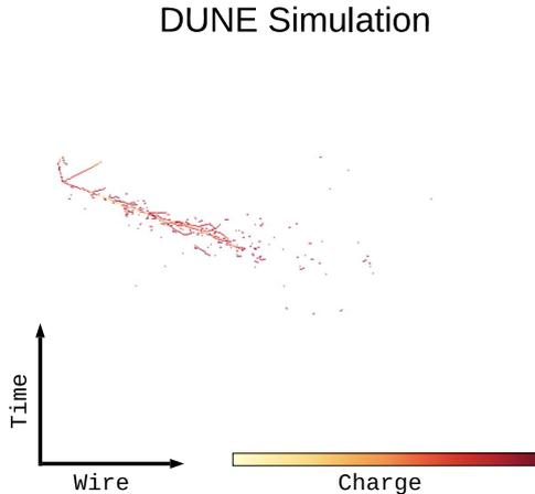
**Fig. 7** A simulated 2.2 GeV  $\nu_e$  CC interaction shown in the collection view of the DUNE LArTPCs. The horizontal axis shows the wire number of the readout plane and the vertical axis shows time. The colorscale shows the charge of the energy deposits on the wires. The interaction looks similar in the other two views. Reproduced from Ref. [70].
