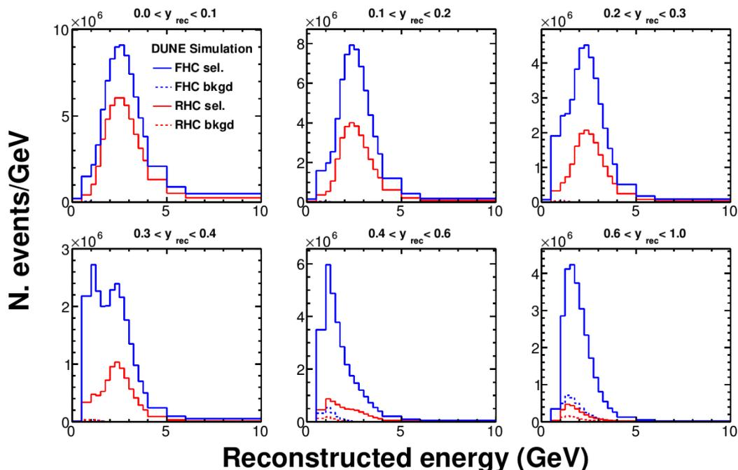
**Fig. 6** ND samples in both FHC (blue) and RHC (red), shown in the reconstructed neutrino energy and reconstructed inelasticity binning used in the analysis. Backgrounds are also shown (dashed lines), which are dominated by NC events, although there is some contribution from wrong-sign  $\nu_\mu$  background events in RHC.
