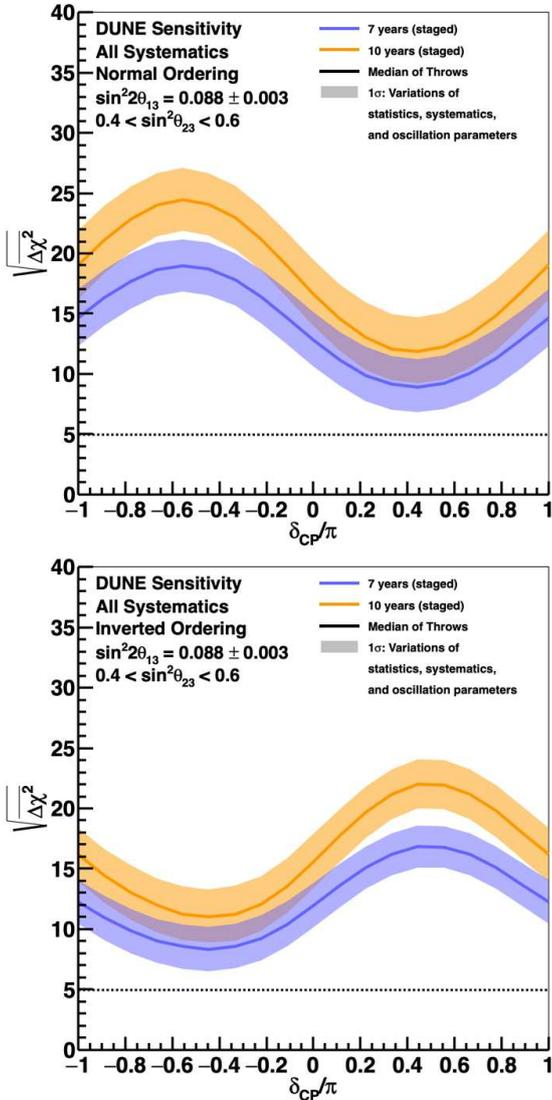
**Fig. 17** Significance of the DUNE determination of the neutrino mass ordering, as a function of the true value of  $\delta_{\text{CP}}$ , for seven (blue) and ten (orange) years of exposure. The width of the transparent bands cover 68% of fits in which random throws are used to simulate statistical variations and select true values of the oscillation and systematic uncertainty parameters, constrained by pre-fit uncertainties. The solid lines show the median sensitivity.
