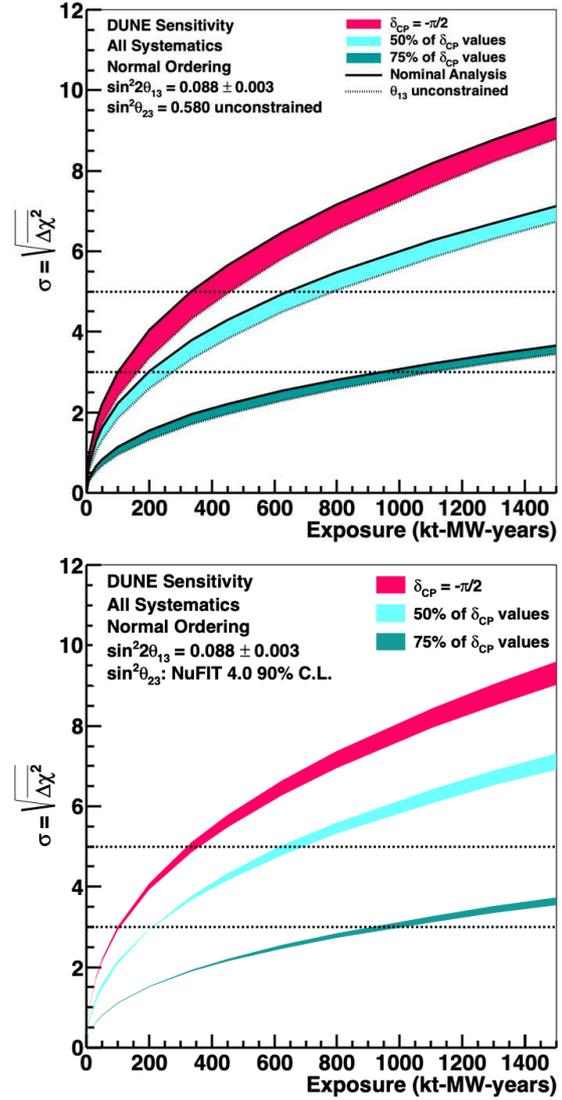
**Fig. 16** Significance of the DUNE determination of CP violation ( $\delta_{CP} \neq [0, \pi]$ ) for the case when  $\delta_{CP} = -\pi/2$ , and for 50% and 75% of possible true  $\delta_{CP}$  values, as a function of exposure in kt-MW-years. Top: The width of the band shows the impact of applying an external constraint on  $\theta_{13}$ . Bottom: The width of the band shows the impact of varying the true value of  $\sin^2 \theta_{23}$  within the NuFIT 4.0 90% C.L. region.
