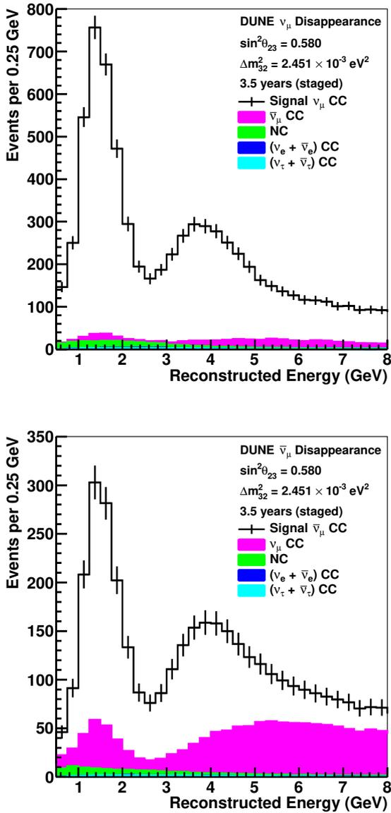
**Fig. 11**  $\nu_\mu$  and  $\bar{\nu}_\mu$  disappearance spectra: reconstructed energy distribution of selected  $\nu_\mu$  CC-like events assuming 3.5 years (staged) running in the neutrino-beam mode (top) and antineutrino-beam mode (bottom), for a total of seven years (staged) exposure. Statistical uncertainties are shown on the datapoints. The plots assume normal mass ordering.
