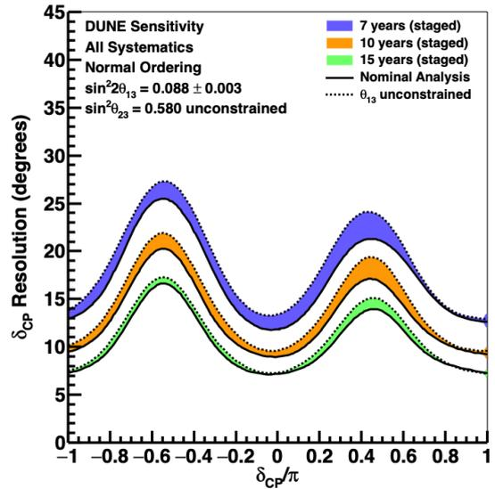
**Fig. 21** Resolution in degrees for the DUNE measurement of  $\delta_{CP}$ , as a function of the true value of  $\delta_{CP}$ , for seven (blue), ten (orange), and fifteen (green) years of exposure. The width of the band shows the impact of applying an external constraint on  $\theta_{13}$ .
