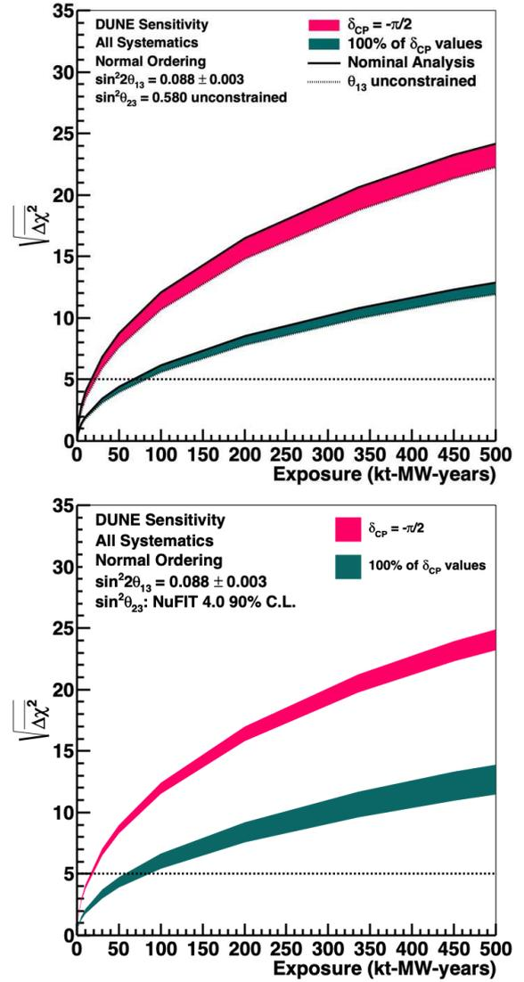
**Fig. 19** Significance of the DUNE determination of the neutrino mass ordering for the case when  $\delta_{CP} = -\pi/2$ , and for 100% of possible true  $\delta_{CP}$  values, as a function of exposure in kt-MW-years. Top: The width of the band shows the impact of applying an external constraint on  $\theta_{13}$ . Bottom: The width of the band shows the impact of varying the true value of  $\sin^2 \theta_{23}$  within the NuFIT 4.0 90% C.L. region.
