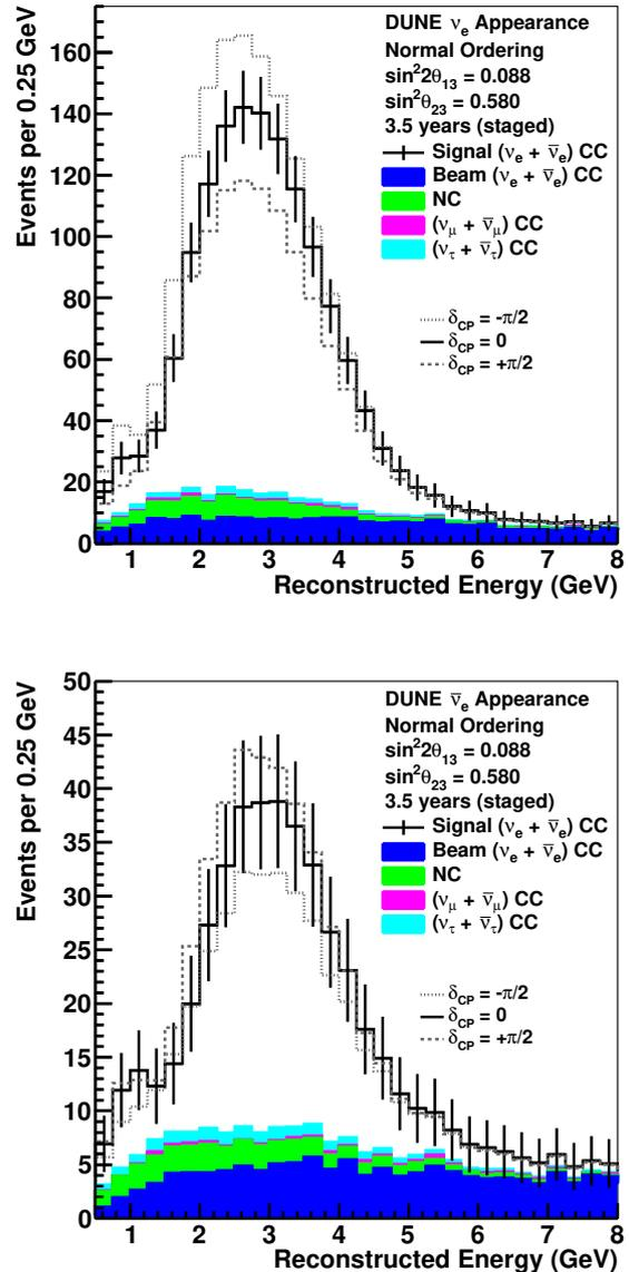
**Fig. 10**  $\nu_e$  and  $\bar{\nu}_e$  appearance spectra: reconstructed energy distribution of selected  $\nu_e$  CC-like events assuming 3.5 years (staged) running in the neutrino-beam mode (top) and antineutrino-beam mode (bottom), for a total of seven years (staged) exposure. Statistical uncertainties are shown on the datapoints. The plots assume normal mass ordering and include curves for  $\delta_{\text{CP}} = -\pi/2, 0, \text{ and } \pi/2$ .
