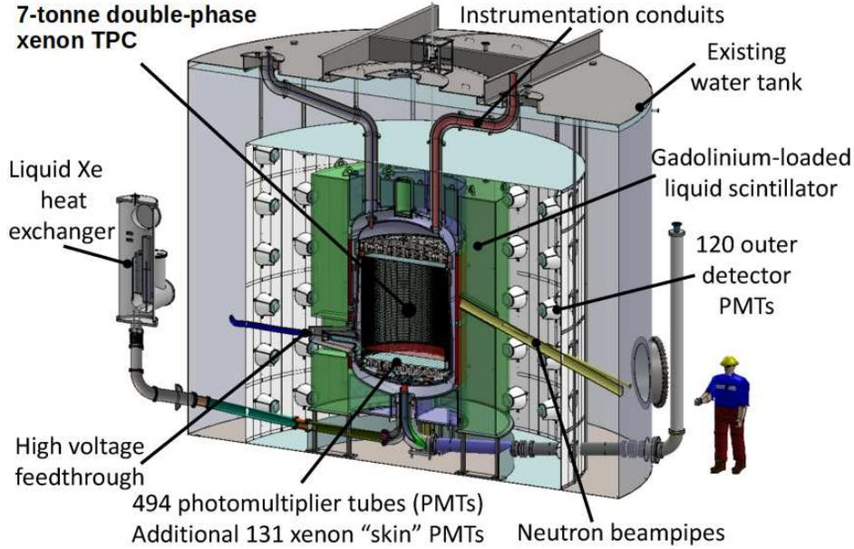
FIG. 1. Cutaway view of the LZ experiment.
