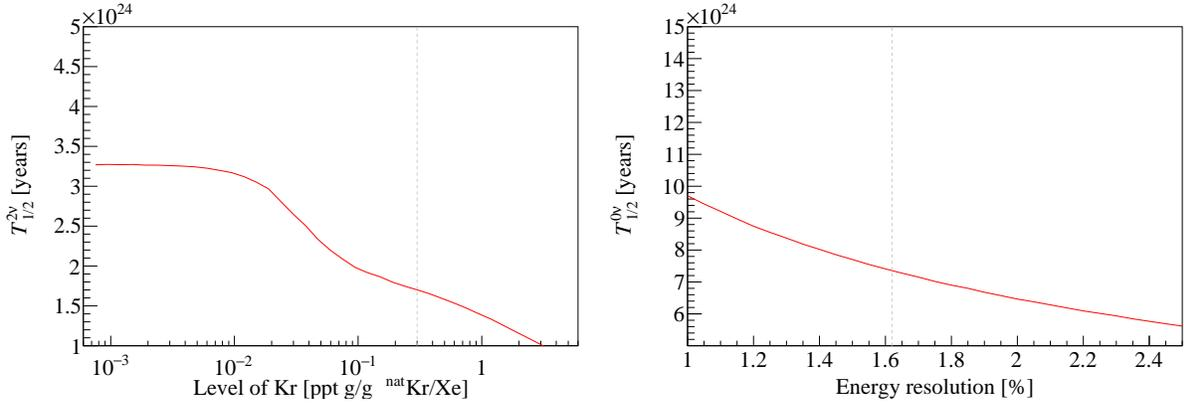
FIG. 5. Dependence of the sensitivity to the  $2\nu 2\beta$  decay of  $^{134}\text{Xe}$  with the level of  $^{85}\text{Kr}$  contamination in LXe (left), and dependence of the sensitivity to the  $0\nu 2\beta$  decay of  $^{134}\text{Xe}$  with the energy resolution at  $Q = 825.8$  keV (right). The gray dashed line indicates the values assumed in this work, namely 0.3 ppt g/g  $^{nat}\text{Kr}/\text{Xe}$  and 1.62%, respectively.
