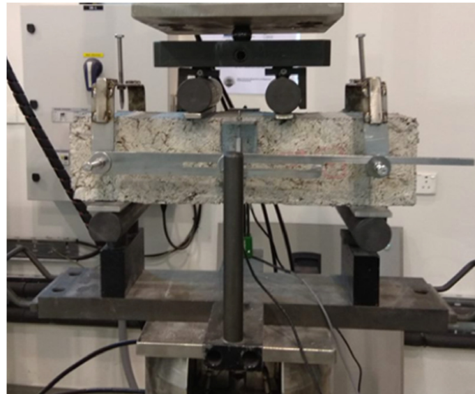
Figure 1. Four-point bending test setup.
