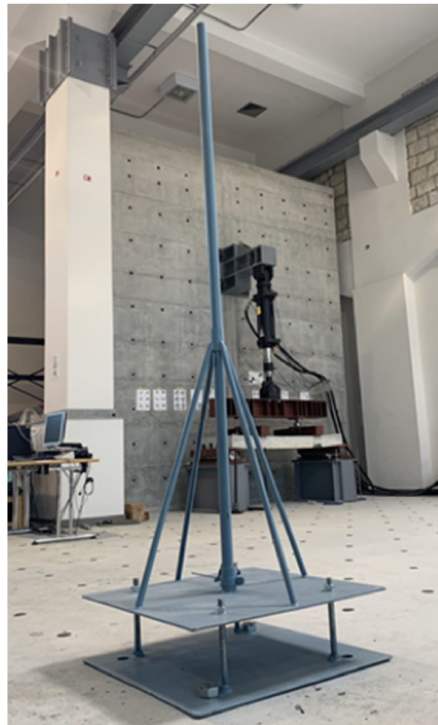
Figure 4. Impact test drop-weight frame.
