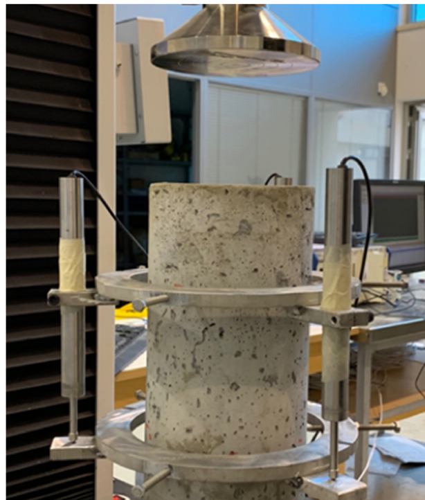
Figure 2. Cyclic compressive loading specimen setup.
