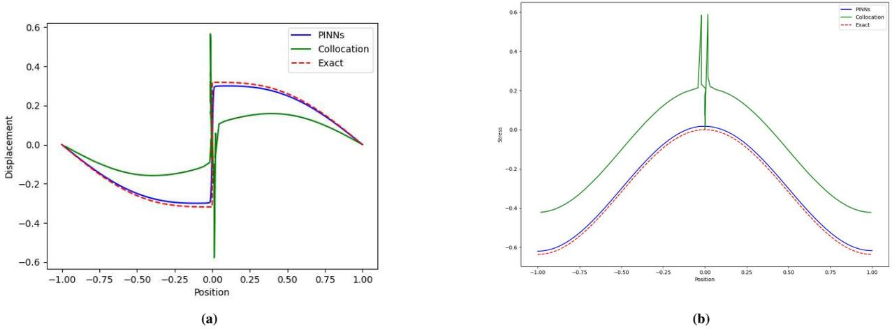
**FIGURE 2** Comparison of displacements (a) and stresses (b) for solutions obtained with PINNs, isogeometric phase-field collocation method and exact solution.
