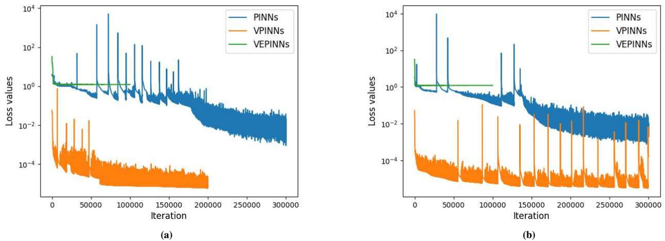
**FIGURE 5** Convergence of the loss functions for (a) a weakly and (b) a strongly imposed Dirichlet boundary condition.
