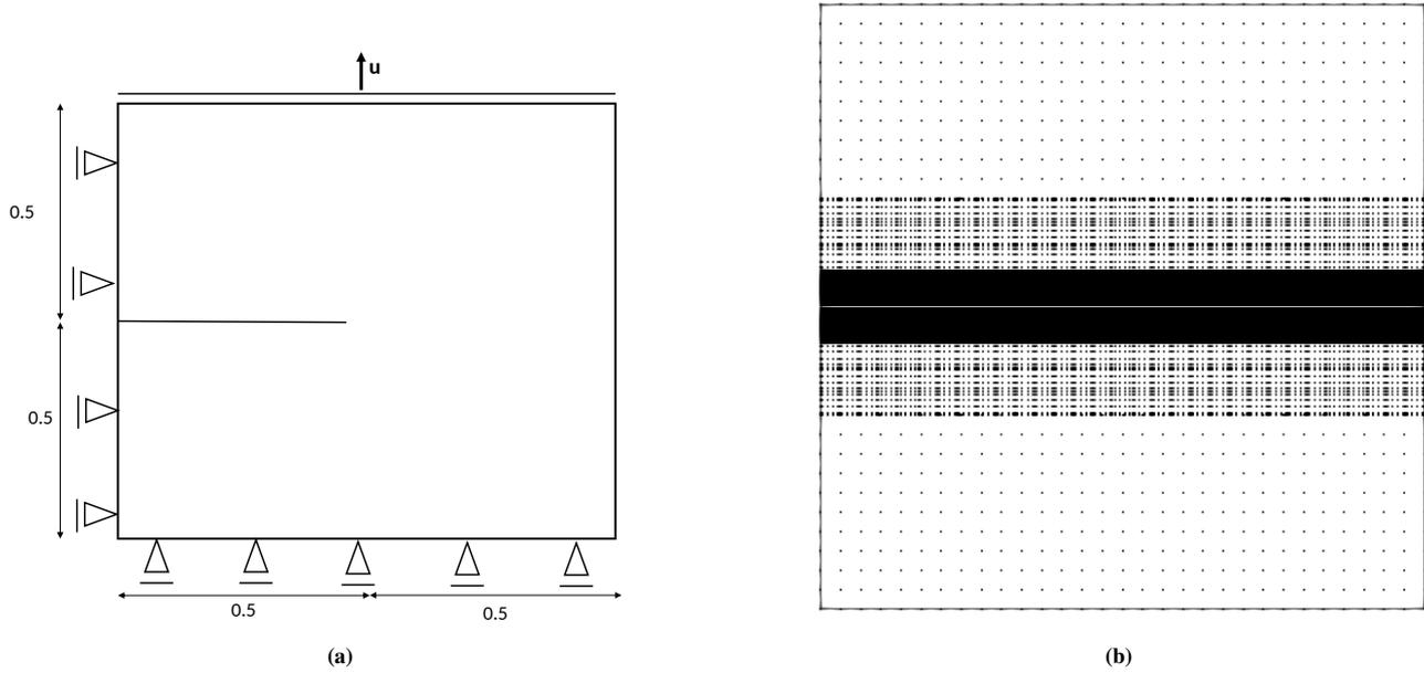
FIGURE 9 a) Geometry and boundary conditions. b) Collocation/integration points distribution
