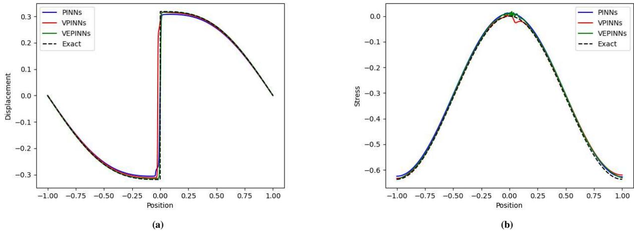
**FIGURE 4** (a) Displacements and (b) stresses with a strongly imposed Dirichlet boundary condition.
