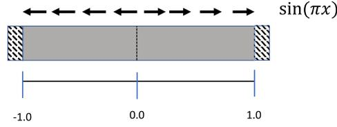
**FIGURE 1** One-dimensional model of a bar with a centre crack under a sinusoidal load
