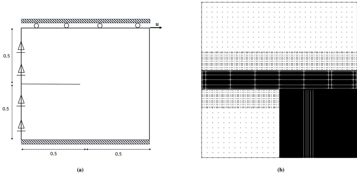
**FIGURE 13** a) Geometry and boundary conditions. b) Collocation/integration points distribution
