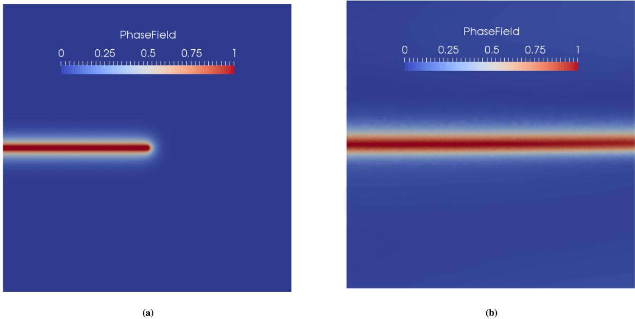
**FIGURE 10** a) Finite element ground truth b) Deep learning prediction with *tanh* activation function; for the prescribed displacement of  $5 \times 10^{-3}$  mm
