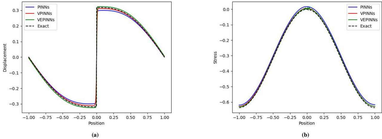
**FIGURE 3** (a) Displacements and (b) stresses with a weakly imposed Dirichlet boundary condition.
