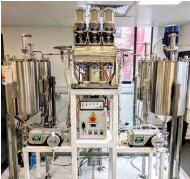
Figure 13: Cascade of 3 stages of 40 mm RD ACCs at the University of Leeds.
