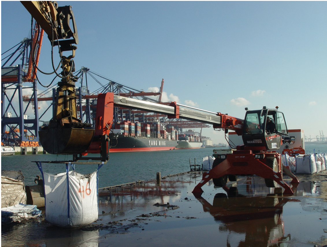
Figure 4 Use of industrial-scale excavation equipment during expansion of the Port of Rotterdam specially designed to obtain grab samples of sediment from the seafloor for archaeological study. The photograph shows a sack filled with sediment recovered from a sand layer at 18 m below sea level that is being lifted clear by a crane mounted on a pontoon. The sediment was then passed through large-scale metal sieves and searched for artefacts and animal bones. Photo by Dimitri Schiltmans, BOOR (Bureau Oudheidkundig Onderzoek Rotterdam), courtesy of Henk Weerts and Hans Peeters.
