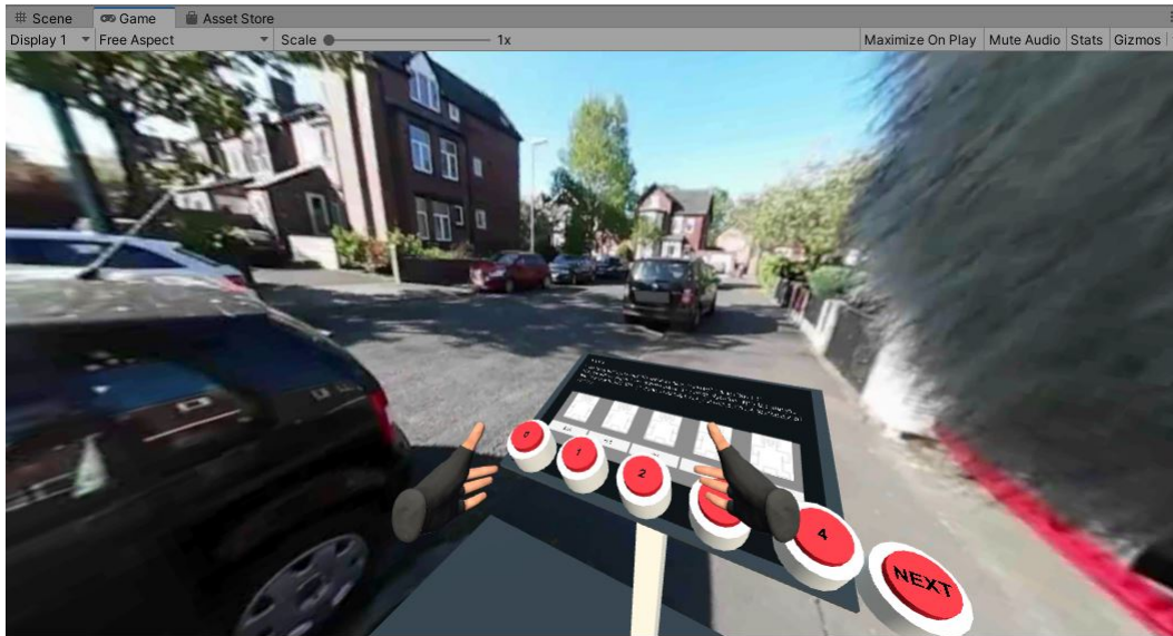
Figure 1: An implementation of a soundscape evaluation experiment as seen through the view of the software development environment. This view would be stereoscopically rendered for a participant wearing a head mounted display system. The view shows the visual stimuli of a 3D still image of a quiet street. The diegetic user interface presented to the participant is also visible, showing a section of the questionnaire and the buttons that participants can use to respond to the questionnaire. Finally the participant hand models are visible.
