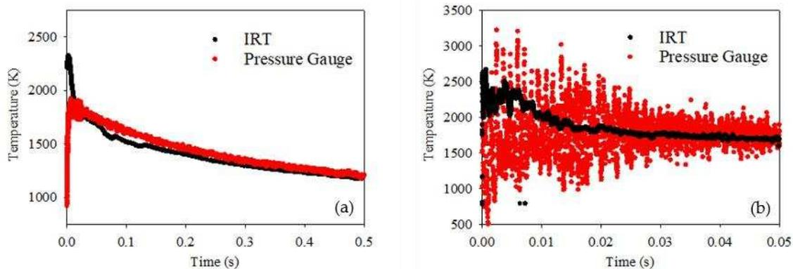
**Figure 7.** Temperature measurement of the confined blast for the (a) first 500 ms of the fireball, with 2 ms filter, and (b) first 50 ms of the fireball, without 2 ms filter.
