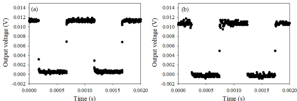
**Figure 4.** Response time assessment of the IRT with a 870 nm LED pulsed with a 1 kHz square wave, measured by (a) the oscilloscope (b) the CompactRio acquisition system.
