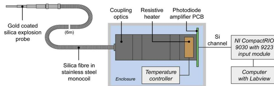
**Figure 1.** Overview of IRT and data acquisition system.
