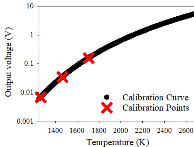
**Figure 5.** Output voltage as a function of temperature for calibrated IRT. Red crosses represent the calibration points at temperatures of 1265, 1463 and 1705 K.
