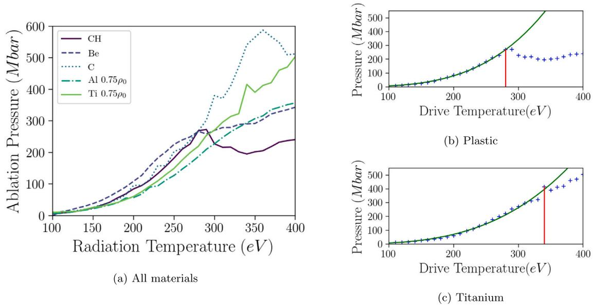
**Fig. 1.** Plots of ablation pressure as a function of drive temperature for (a) all materials. The plots on the right show the results for (b) plastic and (c) titanium. Each cross represents the ablation pressure obtained from an individual simulation performed at a given drive temperature. A suggested maximum drive temperature is indicated by the vertical red line. In (b) and (c), the fitted power laws from Table 1 are plotted as green lines.
