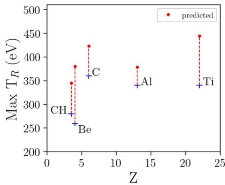
**Fig. 2.** Plots of the approximate maximum drive temperatures for subsonic ablation in the five materials as a function of atomic number,  $Z$ . The red dotted line shows the  $T_{R,critical}$  value predicted by Eq. (8).
