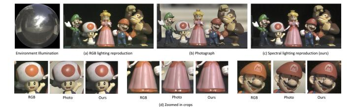
**Figure 1:** Comparison of toy figurines photographed in an outdoor lighting environment (b), and corresponding lighting reproduction inside a multispectral LED sphere using RGB LEDs (a), vs spectral lighting reproduction inside the LED sphere using our proposed spectral upsampling method (c). As can be seen, our RGB-to-spectral upsampling of the input RGB lightprobe achieves a closer qualitative lighting reproduction on the figurines compared to simply driving the LED sphere with RGB values.
