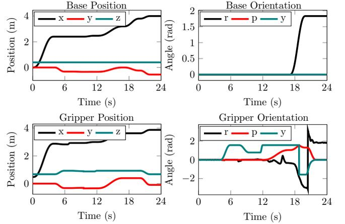
Fig. 3. Planned base and gripper trajectories.
