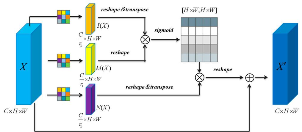
Figure 7. PAB structure diagram.  $\frac{1}{r_1}$  is the channel reduction rate, which can be assigned as  $\frac{1}{2}, \frac{1}{8}, \frac{1}{16}$ .
