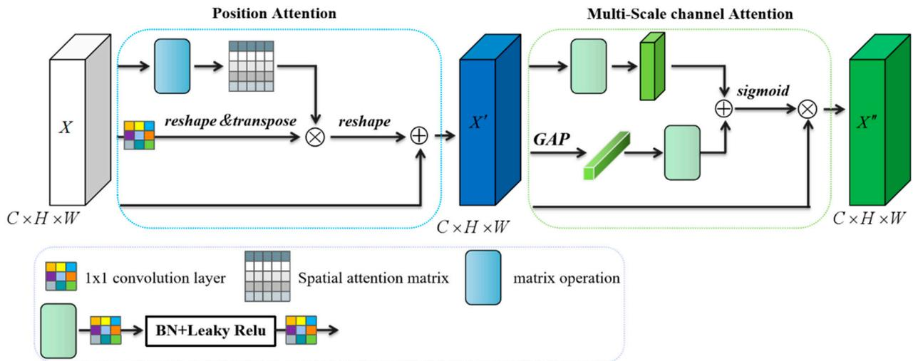
**Figure 6.** Schematic diagram of MSMAM. GAP represents the global average pooling, and BN represents the Batch Normalization.
