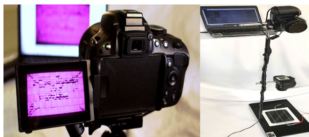
Figure 2. EL imaging setup.
