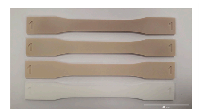
FIGURE 4 | Photo of the equivalent part from all three builds containing the custom additives and one without additives. Shown are (top to bottom), virgin PA2200 + 1% P50, virgin PA2200 + 1% P45, virgin PA2200 + 1% P40, virgin PA2200.
