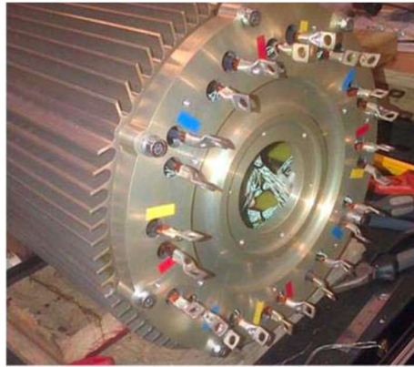
Figure 1. A fin-cooled electric tail motor [19].
