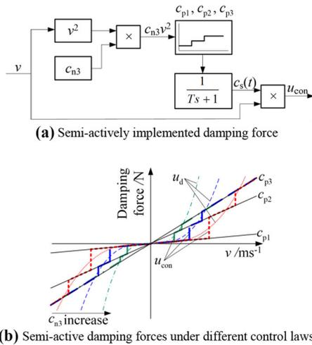
**Fig. 10** The semi-actively implemented nonlinear damping force
