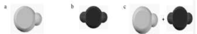
Fig. 3. (a) a two-particle clump used to develop model 1, (b) a 3-particle clump used to develop model 2 and (c) a mixed particle clump used to develop model 3.
