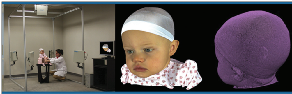
Figure 2: Left: the 3dMDhead system with five 3D cameras arranged to capture the human head. Center: view of the 3D image with color-texture applied to the 3D mesh. Right: raw 3D point cloud from infrared-based active stereo
