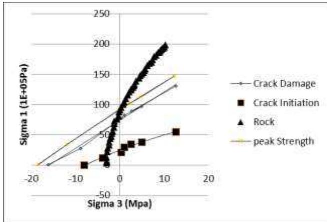
Fig. 7. Rock strength, Crack Initiation, Crack Damage and Peak Strength at 20MPa Confined Pressure for Ughelli sandstone under triaxial compression
