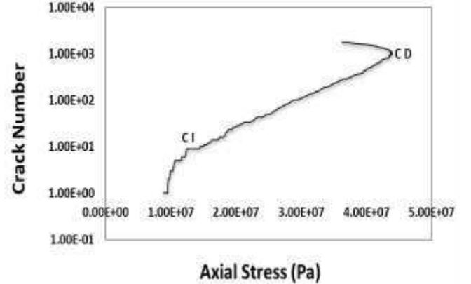
Fig. 3. Crack Initiation (CI) and crack damage (CD) stresses for unconfined axial stress application. The crack number are limited to  $(1 \times 10^4)$  particles used for building sandstone sample in the Discrete Element Modelling (DEM).
