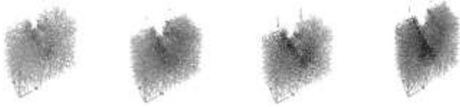
Fig. 4. Force chains of stress transmission during loading at 0.4N, 0.8N, 1N and 2N. The lighter colored force chains are compression while dark colored force chains are tension
