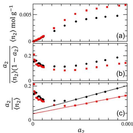
**Figure 6.** The low  $a_2$  behavior of the argon adsorption on crystalline (red) and pelleted (black) zeolite 13X using the data published by Pini at 87 K.<sup>38</sup> (a) Adsorption isotherms. (b) The BET plot (eq 14b) which exhibits a negative gradient at  $a_2 \rightarrow 0$ . (c)  $\frac{a_2}{\langle n_2 \rangle}$  plot with the fitting equation (eq 13 with  $C_0 = 0$ ) using data between  $a_2 = 4 \times 10^{-4}$  and  $1 \times 10^{-3}$ .
