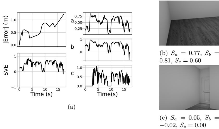
Fig. 3: (a) shows the visibility outputs from ORB-SLAM2 SVE for trajectory ‘original\_3.3’ in the ‘3FO4K7I2Q0PG’ subset of the InteriorNet dataset. (b) shows the image frame with the highest associated visibility ( $t \approx 4$  s) (c) shows the frame with the lowest associated visibility ( $t \approx 9.19$  s)
