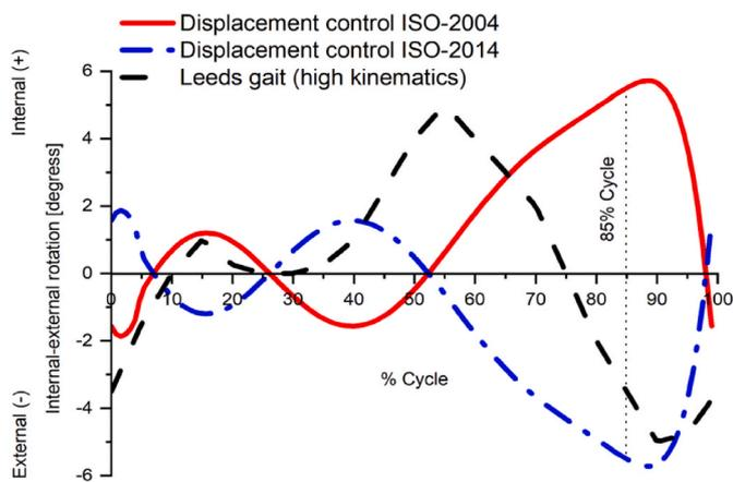
**Fig. 2.c.** Tibial rotation input profiles for different displacement controlled test methods (ISO-14243-3, 2014, McEwen et al., 2005; Barnett et al., 2001, ISO-14243-3, 2004).
