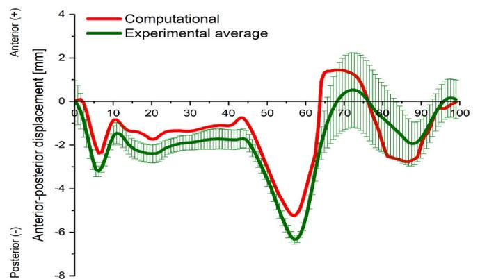
Fig. 7. Computationally predicted AP displacements [mm] compared to experimental AP displacements [mm] (mean ± 95% CI, n = 100 cycles) using the force control ISO-2009 input kinematics.
