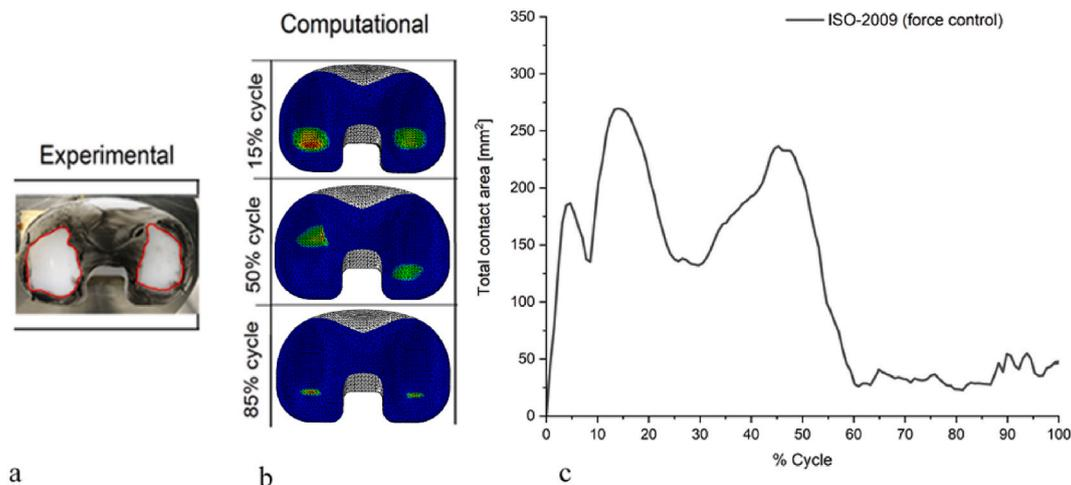
**Fig. 10.** (a) Experimental total contact scars, (b) computational contact scars at 15%, 50%, and 85% through the gait cycle, (c) computational total contact areas at different points through the gait cycle using ISO-14243-1-2009 force control test method.
