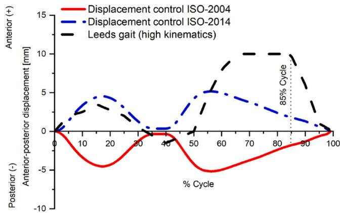
**Fig. 2.b.** Anterior-posterior displacement input profiles for different displacement controlled test methods (ISO-14243-3, 2014, McEwen et al., 2005; Barnett et al., 2001, ISO-14243-3, 2004).
