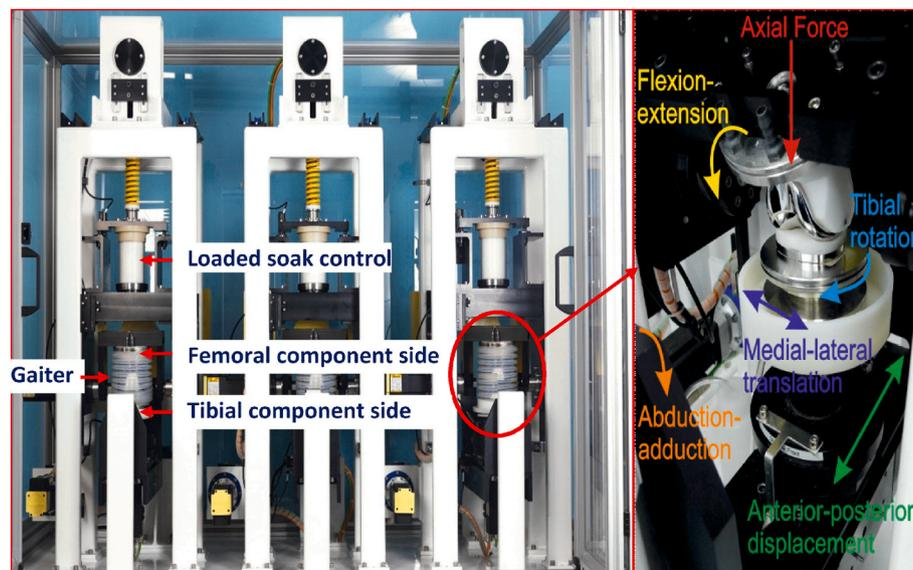
Fig. 1. Six station electromechanically driven knee simulator (Simulation Solutions, UK), and the six degrees of freedom for each station.
