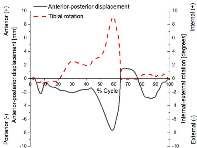
**Fig. 9.** Computationally predicted anterior-posterior displacement [mm] and tibial rotation angle [degrees] of the lowest point of the medial condylar using ISO-14243-1-2009 force control test method.
