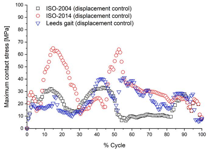
Fig. 5. Computationally predicted maximum contact stress [MPa], at different percentages through the gait cycle, for different displacement control test methods.
