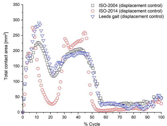
Fig. 4.c. Computational total contact areas at different points through the gait cycle using different displacement control test methods.
