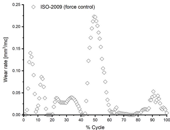
Fig. 12. Computationally predicted wear rate [ $\text{mm}^3/\text{million cycles}$ ], at different percentages through the gait cycle, for ISO-14243-1-2009 force control test method.
