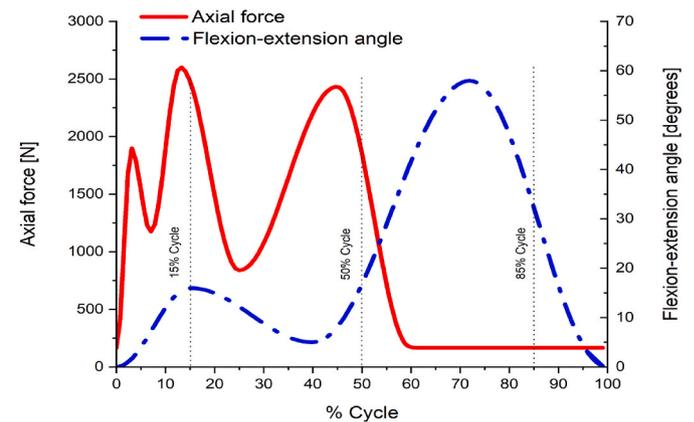
Fig. 2.a. Axial force and flexion-extension angle input profiles for all test methods.
