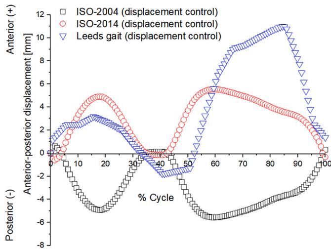
Fig. 4.d. Computationally predicted anterior-posterior displacement [mm] of the lowest point of the medial condyle using different displacement control test methods.
