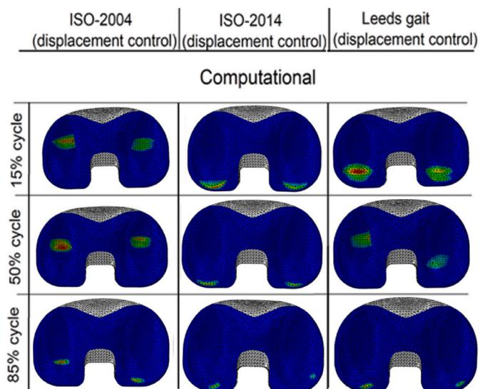
Fig. 4.b. Computational contact scars at 15%, 50%, and 85% through the gait cycle using different displacement control test methods (more points throughout the cycle are openly available through the University of Leeds data repository (Abdelgaied and Jennings, 2022)).
