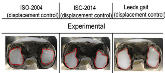
Fig. 4.a. Experimental total contact scar areas using different displacement control test methods.
