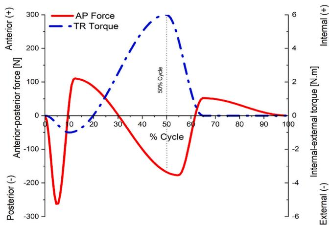
**Fig. 3.** Anterior-posterior force and internal-external tibial rotation torque input profiles for the ISO force controlled test method (ISO-14243-1, 2009, ISO-14243-3, 2014).
