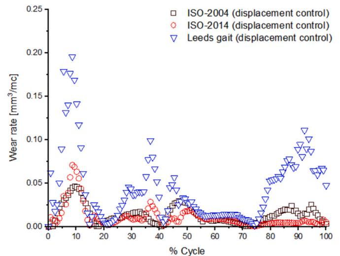
Fig. 6. Computationally predicted wear rate [mm<sup>3</sup>/million cycles], at different percentages through the gait cycle, for different displacement control test methods.
