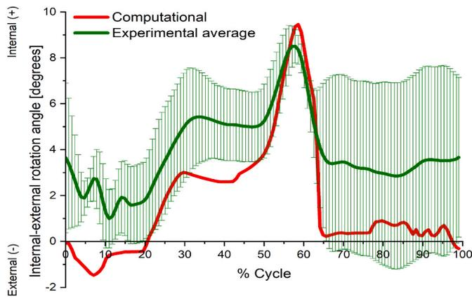
**Fig. 8.** Computationally predicted tibial rotation angle [degrees] compared to experimental tibial rotation angle [degrees] (mean  $\pm$  95% CI, n = 100 cycles) using the force control ISO-2009 input kinematics.
