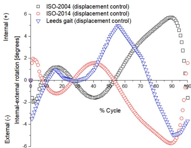
Fig. 4.e. Computationally predicted tibial rotation angle [degrees] of the lowest point of the medial condyle using different displacement control test methods.
