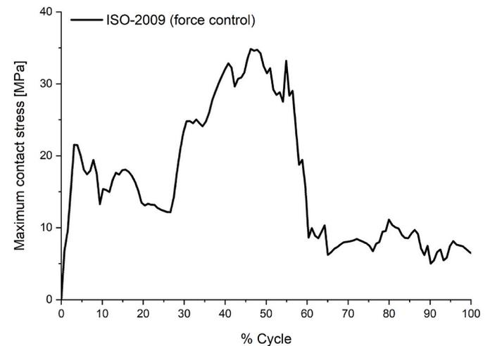
**Fig. 11.** Computationally predicted maximum contact stress [MPa], at different percentages through the gait cycle, for ISO-14243-1-2009 force control test method.
