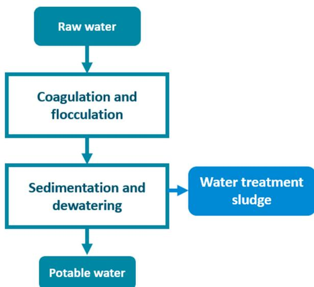
Fig. 5. Block-flow diagram of a water treatment process.
