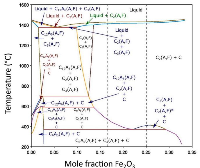
Fig. 7. Isopleth in the  $\text{CaO}-\text{Fe}_2\text{O}_3-\text{Al}_2\text{O}_3$  ternary diagram in air ( $p(\text{O}_2) = 0.21$  atm) where  $x(\text{CaO}) = 0.6667$  showing ferrite  $\text{C}_2(\text{A},\text{F})$  stability calculated using Thermo-Calc 2020b software and OXDEMO: Oxide demo database v2.0.
