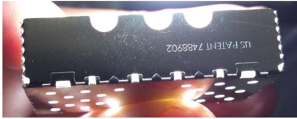
Fig. 13. Shield 1 with back illuminations showing gaps.
