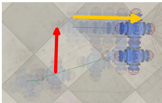
Figure 6. Docking of a robot to a moving seed, note how, while in the global reference frame, the recruited robot follows an angled path, from the reference frame of the recruiter it is simply approaching while keeping aligned to the cone's centre.
