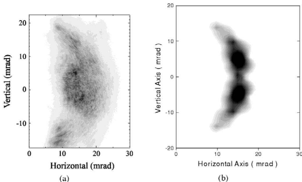
**Fig. 1.** The far-field Ne-like Ge X-ray laser output at 19.6 nm produced with double 75-ps optical pulses (a) measured with an imaging multilayer mirror and CCD and (b) simulated using the EHYBRID and ray trace codes.
