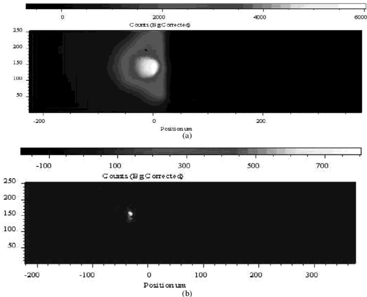
**Fig. 2.** Beam profiles of a Ne-like Ge laser at 19.6 nm at a distance of 1.6 cm from a 4-mm length of density well target of (a) copper and (b) germanium. The profile after passing through the germanium is spatially smaller, but much less intense. The relative but comparable intensity scales are indicated above the respective plots (light shading is more intense).
