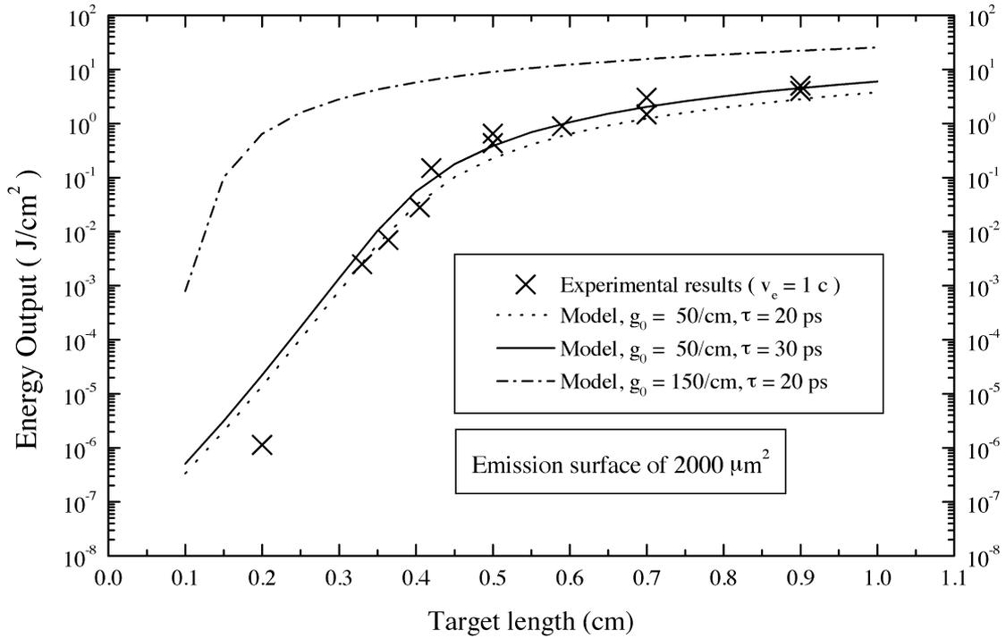
**Fig. 6.** X-ray laser output at 19.6 nm for Ne-like Ge pumped with approximate picosecond pulses and travelling wave excitation along the target length. Model results with the parameters shown are also plotted as curves.
