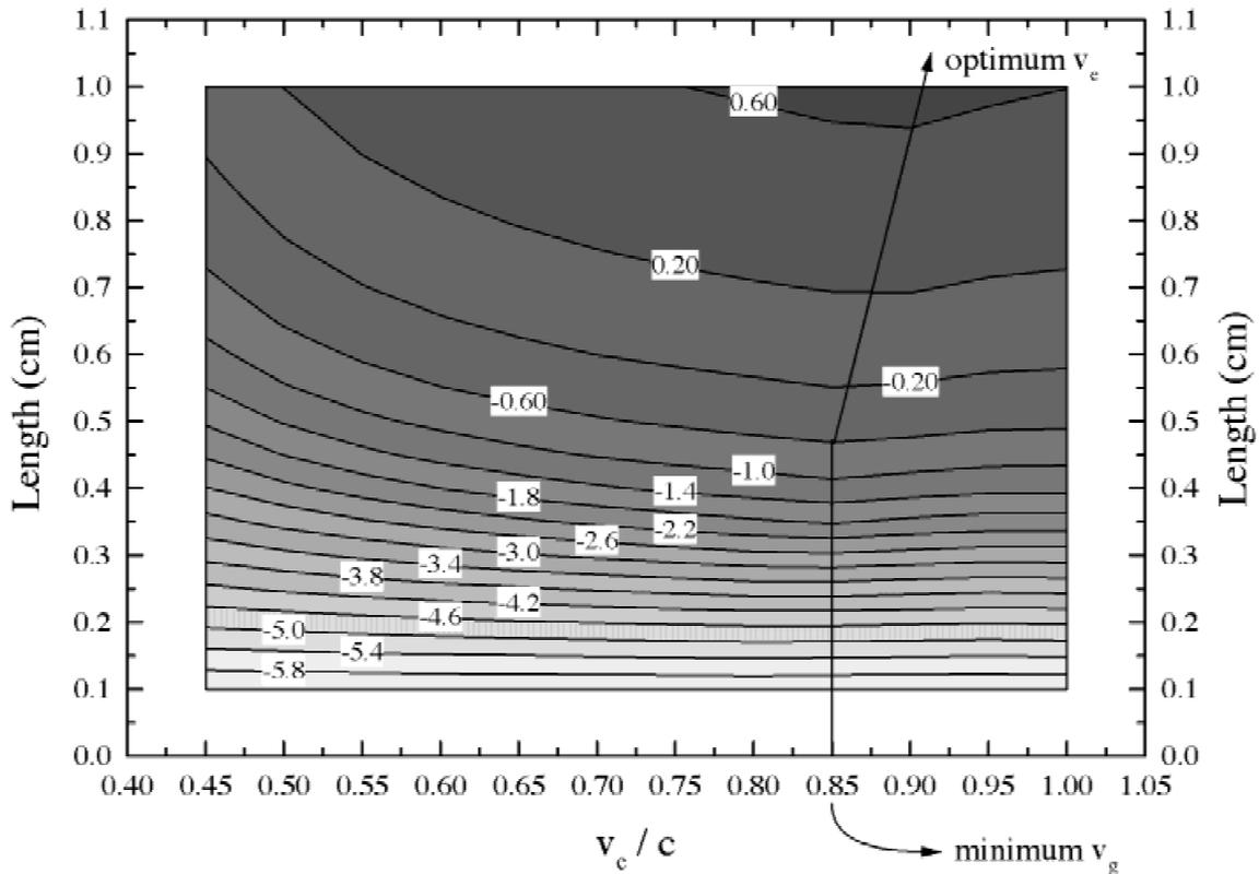
**Fig. 7.** X-ray laser output in units of  $\text{Jcm}^{-2}$  plotted as contours on a base10 logarithmic scale as a function of target length and excitation speed along the target. The calculations are for gain coefficient  $50 \text{ cm}^{-1}$ , gain duration 20 ps, spectral bandwidth  $\sim \nu/\Delta\nu = 10^4$ , saturation flux  $2 \times 10^{10} \text{ Wcm}^{-2}$  and “spontaneous emission” of  $2 \times 10^3 \text{ Wcm}^{-2}$ .
