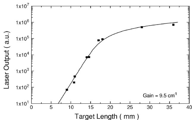
**Fig. 3.** The variation with length of the output of Ni-like Sm at 7.3 nm pumped with double 75-ps pulses. The gain coefficient of  $9.5 \text{ cm}^{-1}$  is obtained by fitting the Linford formula to the approximately exponential increase in output at shorter target lengths.
