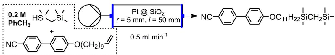
**Figure 5:** Continuous flow hydrosilylation of 4'-(11-hydroxyundecyloxy)-4-cyanobiphenyl and 1,1,3,3-tetramethyldisilabutane using a platinum-on-silica catalyst ("Pt @ SiO<sub>2</sub>").
