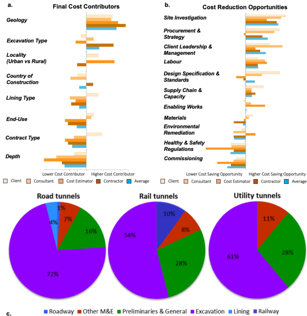
Figure 2. (a) Cost Contributors in tunnelling projects, (b) cost reduction opportunities and (c) breakdown of construction cost composition (modified from [35]).
