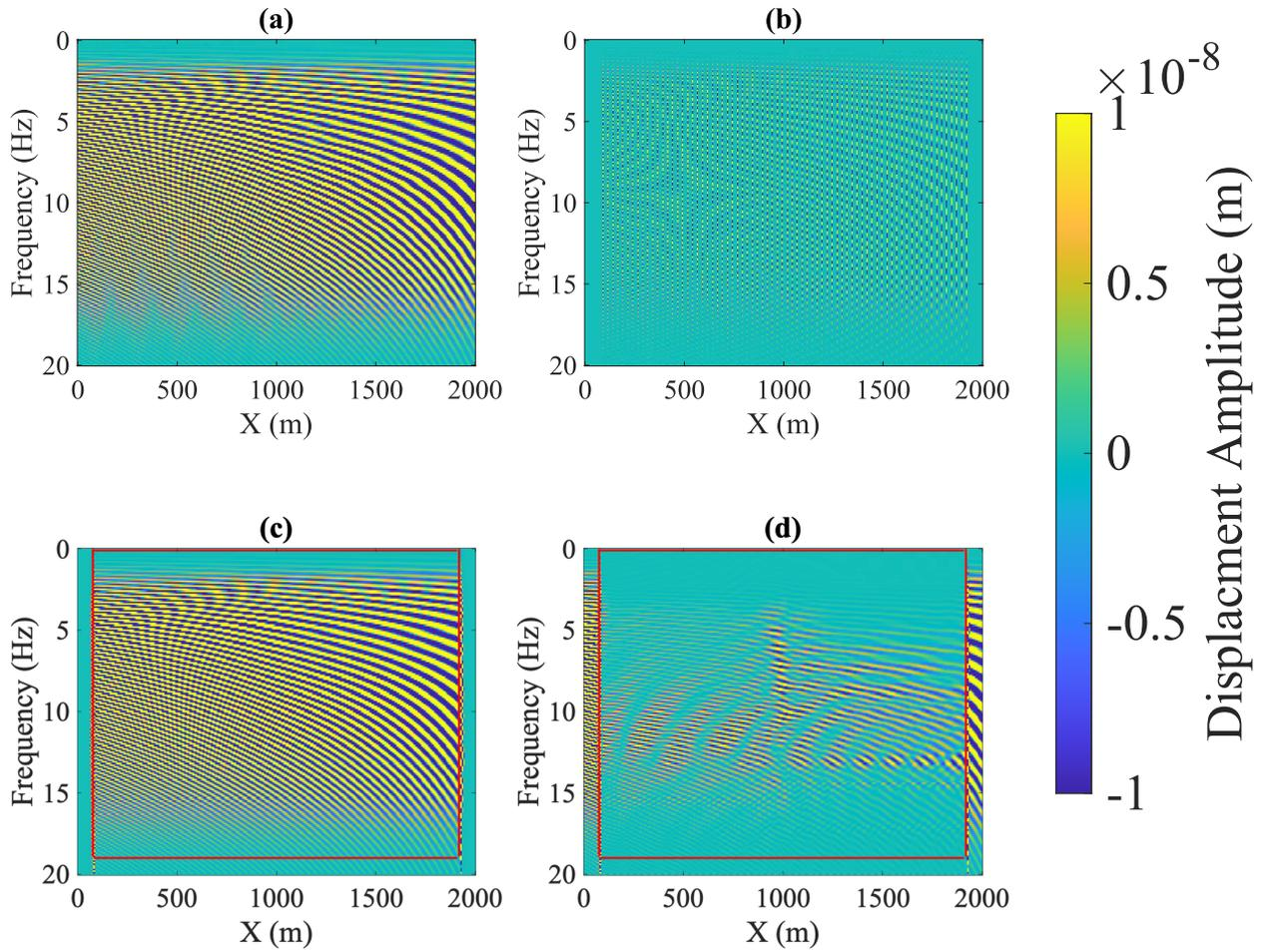
**Figure 3.** FWFI wavefield results for an active seismic scenario. a) True modelled wavefield in the space-frequency domain as obtained from the first scenario in Fig. 2a. b) The decimated data input to WFI sampled every 25 m. c) Wavefield estimated by FWFI after 50 iterations. d) Difference between true and estimated wavefields. The red box in (d) shows the zone where we inverted for phase velocities. Note, spatial sampling intervals are 5 m in panels a, c and d, and 25 m in panel (b).
