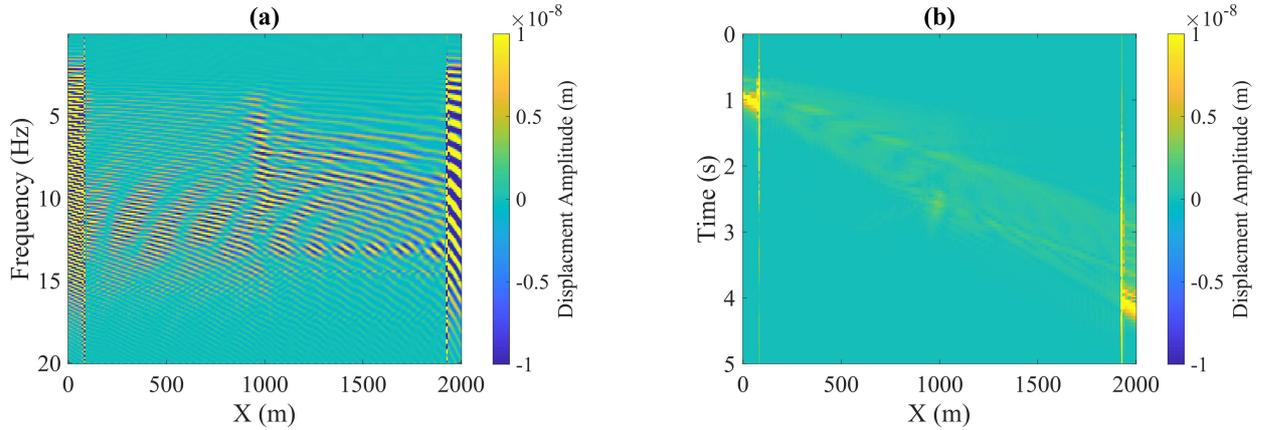
**Figure 4.** Difference between true and estimated wavefields in frequency domain (a) which transformed to time domain (b).
