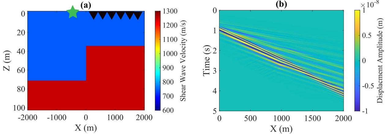
**Figure 2.** Acquisition geometry and modelling results. a) Is the shear velocity model we used to generate experimental data. The star shows the seismic source while the triangles show the location of the receiver array. b) The elastic modelling result in the time domain for the acquisition scenario in (a). The amplitude is proportional to the source function.
