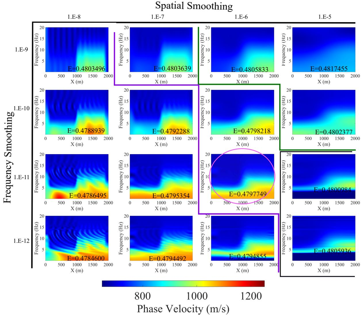
**Figure 6.** Velocity properties obtained using different combinations of both spatial and frequency smoothing scaling parameters  $\epsilon_2$  and  $\epsilon_3$ , respectively. We choose the circled combination as it has the lowest  $E$ , data residual, among the remaining combinations. For definitions of purple, green and black curves refer to the main text.
