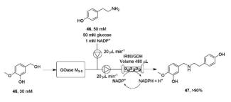
Scheme 18 Flow system for the oxidation-reductive amination cascade towards the synthesis of 4-O-methyl norbelladine  $47.^{77}$
