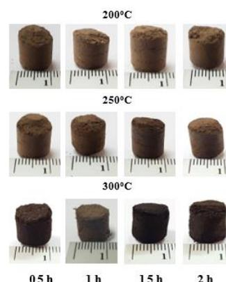
Figure 4. Torrefied fuel pellets (compression pressure 30 bar)
