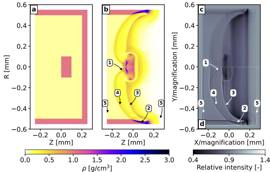
**Fig. 8.** Shock interaction: a) density map in the plane  $ZR$  at time 0; b) density map 7 ns after the beginning of the laser ablation; c) XACI image of the object showed in b); d) XPCI image of the same object. Labels: 1) collapsed shock; 2) sheared flow; 3) interface matter-vacuum; 4) main shock; 5) interface plastic-foam.
