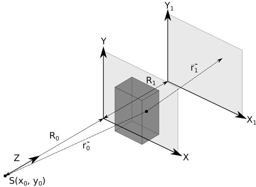
**Fig. 2.** Visualization of the geometry. The object (dark gray box) is placed at a distance  $R_0$  from the source  $S$  and  $R_1$  from the image plane  $(X_1, Y_1)$ . The X-ray beam propagates along the  $Z$ -axis, which is perpendicular to the object and image plane.
