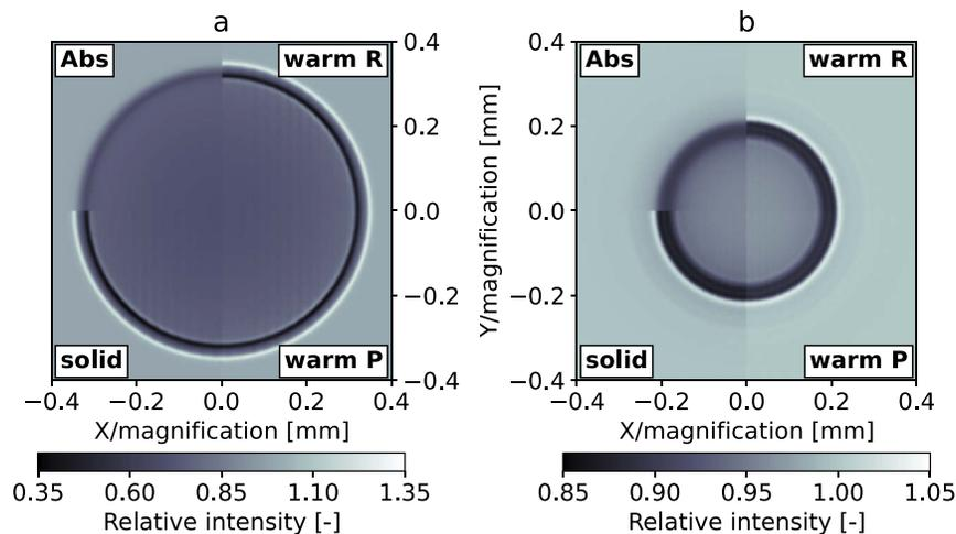
**Fig. 5.** Spherical implosion: XACI and XPCI images for the plastic sphere (a) and the shell (b). For each image: *Abs* is the pure attenuation image, *warm R* XPCI using Rosseland opacity, *warm P* XPCI using Planck opacity, *solid* XPCI using solid-cold model.
