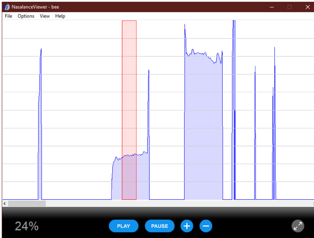
Fig. 4. Screenshot of the Nasalance Viewer software demonstrating the calculation of nasalance within a marker region. The region corresponding to the portion used in the first take of ‘bee’ for normal speech is shown in red; the average nasalance within the region is shown in the bottom left corner.
