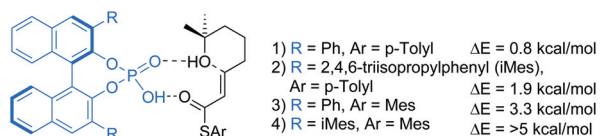
Fig. 1 Preliminary computational study of a CPA catalysed enantioselective oxa-Michael reaction. MMFF energy differences between lowest S and R producing TS-like structures shown in kcal mol -1 . S product favoured in all cases.
