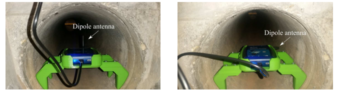
Fig. 4. Two different orientations used for the transmitter and receiver dipole antennas. Also pictured a Pluto SDR unit in its holder.
