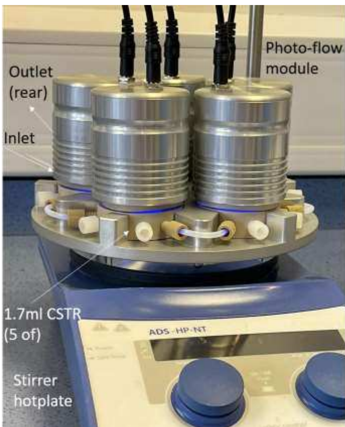
Figure 1: Arrangement of the photo-flow modules on the individual CSTRs. Here, a complete set of five modules in series are shown.
