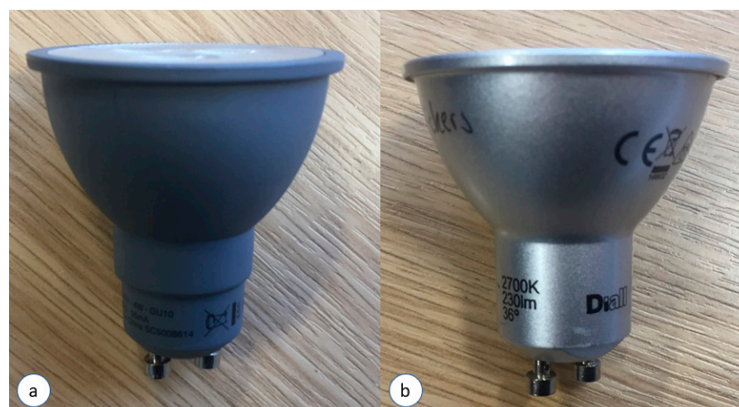
Figure 1. Two failed LED spotlights with GU10 socket. Sample A (a) does no longer emit any light, Sample B (b) flickers.
