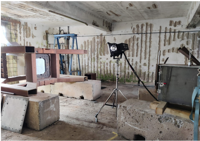
Figure 9 Photograph of the blast test arrangement prior to detonation
