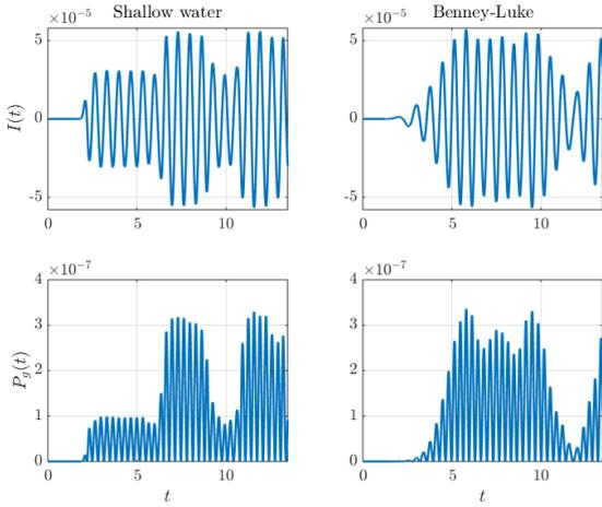
Fig. 4. Generated current  $I$  (in Ampere) and power  $P_g$  (in Volt×Ampere) as functions of time  $t$  (in seconds), obtained in the case of shallow water (left-hand panels) or from the Benney-Luke system (right-hand panels).
