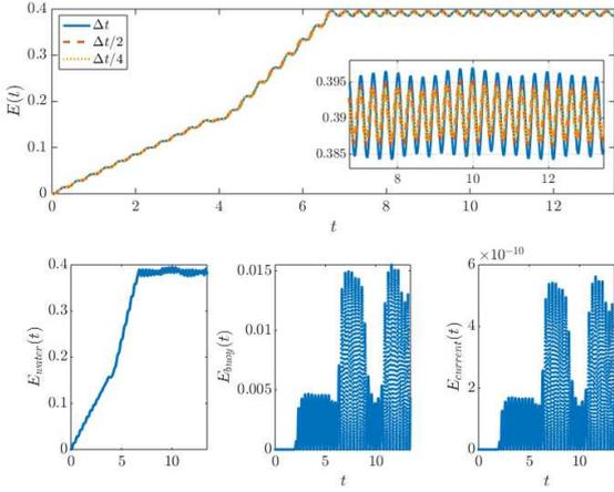
Fig. 6. Energy evolution over time  $t$  (in s) for overall energy  $E$  and energies  $E_{water}$ ,  $E_{buoy}$  and  $E_{current}$  (all in J) of the three subsystems for a shallow-water simulation. Mean energy for  $t > T_w$  is 0.39J.  $A = 0.0653\text{m}$  and  $\omega = 9.33\text{Hz}$ . Energy for time-steps  $\Delta t, \Delta t/2, \Delta t/4$ ;  $N_x = 10, N_y = 50$ . (Inset panel shows time convergence).
