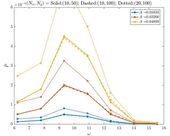
Fig. 9. Generated power (in Volt×Ampere) as function of wave-maker frequency  $\omega$  for three wavemaker amplitudes  $A$  for the dispersive linearised Benney-Luke system, over  $T = 10\text{s}$ . Resonance at circa 9.33Hz. The solution eventually diverges.
