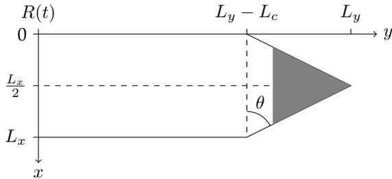
(b) Top view of the tank and buoy, outlining the tank's dimensions and how the buoy fits the shape of the contraction.
