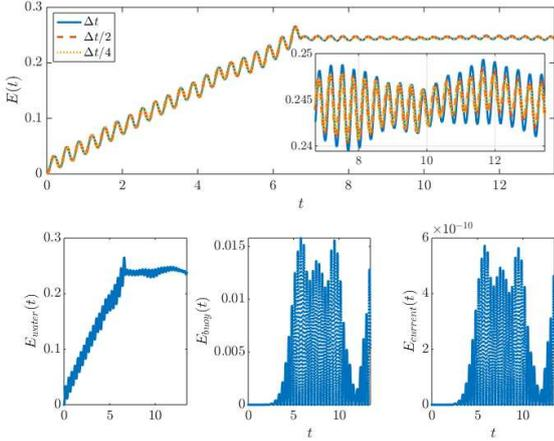
Fig. 7. Energy evolution over time  $t$  (in s) for overall energy  $E$  and energies  $E_{water}$ ,  $E_{buoy}$  and  $E_{current}$  (all in J) of the three subsystems for a BL-simulation. Mean energy for  $t > T_w$  is about 0.245J.  $A = 0.0653\text{m}$  and  $\omega = 9.33\text{Hz}$ . Energy for time-steps  $\Delta t, \Delta t/2, \Delta t/4$ ;  $N_x = 10, N_y = 50$ . (Inset panel shows time convergence).
