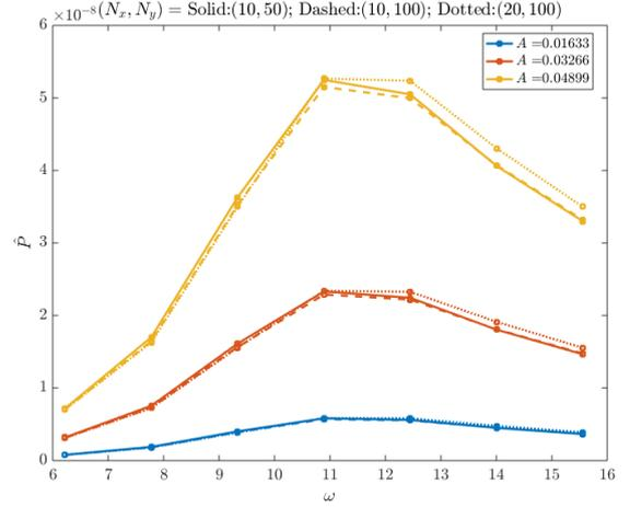
Fig. 8. Generated power (in Volt×Ampere) as function of wave-maker frequency  $\omega$  for three wavemaker amplitudes  $A$  for the non-dispersive linearised shallow-water system, over  $T = 10\text{s}$ , at various resolutions. Resonance at circa 11Hz.
