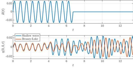
Fig. 3. Wavemaker output and free surface evolution (in m) at  $y = 0$  as function of time  $t$  (in s). The wavemaker is on for  $T_w = 10$  periods and then switched off with time shown for  $2T_w$ . The fastest, shallow-water reflected waves arrive back at the wavemaker at approximately  $t = 4$ s but due to dispersion slowing down shorter waves this is less prominent in the BL-system.  $A = 0.0653$ m and  $\omega = 9.33$ Hz.
